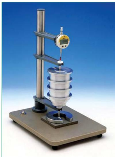
Results are displayed on a digital indicator gauge that automatically zeros at the press of a button.
