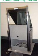
The WIRA Flammability Tester is used to test the effects of a small source of ignition on floorcoverings. It can be used for either the hot metal nut test (BS 4790) or the methenamine tablet test (ISO 6925 and BS 6307).
