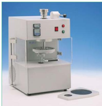
a screw clamp. The number of rubs (revolutions) required for a test can be set on a predetermining counter and the number carried out is shown on a totaliser. Another counter displays the total number of rubs in successive testing cycles.
