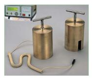
A versatile megohmeter for the measurement of resistance to earth of textile based floorcoverings. Suitable for laboratory or production testing and compliant with BS7078:1989. The front panel pass/fail lamps permit easy and fast evaluation of measurements. The memory function enables up to 10 set configurations to be stored.
