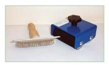
The Pilfuz Carpet Test is used to simulate the "fuzz" and pill that can be associated with carpets under normal use.
